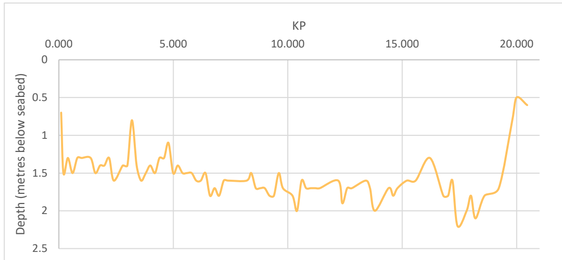
Figure 2-4 Wingate Pipelines Depth of Burial (2013)
