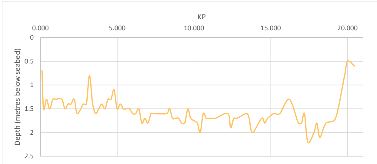
Figure 1-3 Wingate Pipelines Depth of Burial (2013)
